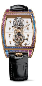
MOVEMENT CO IOO - Hand-wound 90 hours power-reserve Functions: Hours, minutes, flying tourbillon, small seconds with the tourbillon cage Frequency: 3 Hz, 2I,600 vph Dimension: 20" x I3 34"" Sapphire crystal plate and bridges
